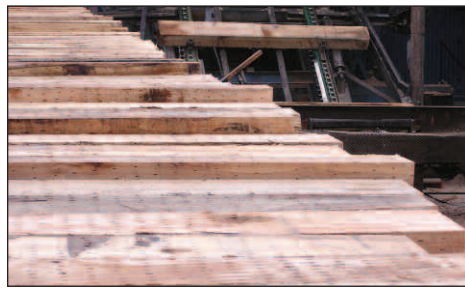
Untreated ties arrive and are sorted and stacked to air dry prior to treatment.
