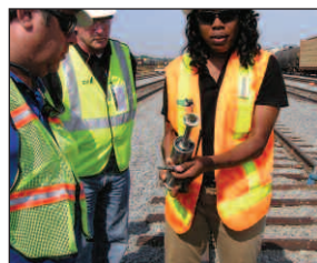
Joules (piston) "retarders" are strategically placed throughout the 45 different tracks to maintain each car's speed at 6, 4, and 2 mph. These upgrades have resulted in increased efficiency and decreased cost.
