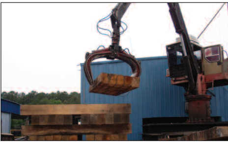
Untreated ties arrive and are sorted and stacked to air dry prior to treatment.
