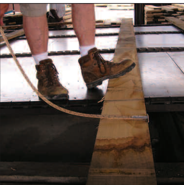
A Miller Lumber supervisor uses a hickory measurement tool to grade and record their product.
