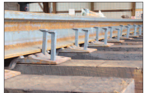
This Koppers plant also prepares 40-foot track panels with 24 ties attached to track sections in advance.
