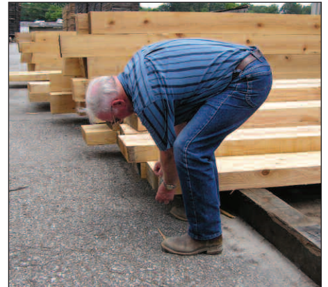
Harry Bressler (Stella-Jones/BPB) uses the dollar bill measuring test.
