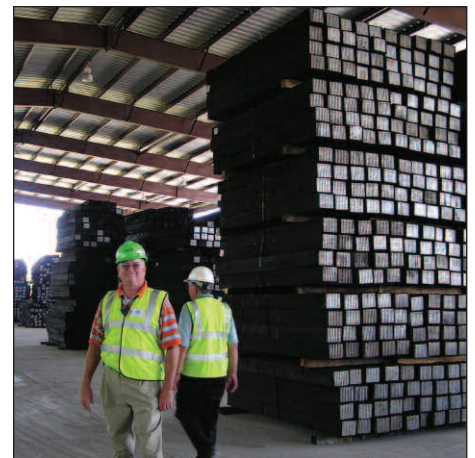
Production Manager Joe Fields explains how the treated ties are housed under cover and then loaded onto cars for transport.
