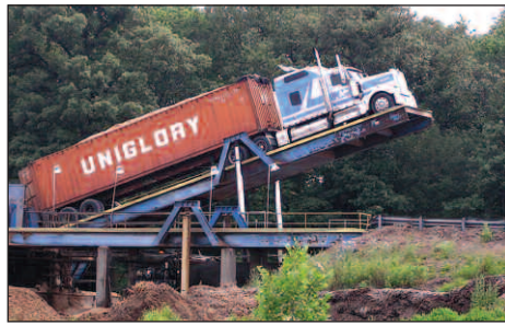
Wood chips arrive at the New Johnsonville, Tenn., plant in container cars that are pulled onto the receiving platform. The entire truck is raised to let the chips fall into the collection bin and off to processing.
