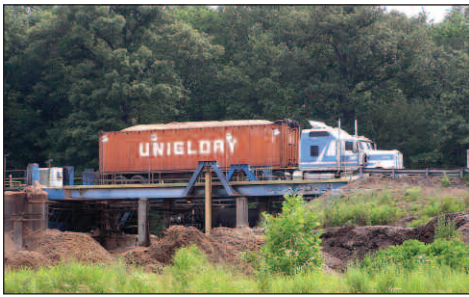
Wood chips arrive at the New Johnsonville, Tenn., plant in container cars that are pulled onto the receiving platform. The entire truck is raised to let the chips fall into the collection bin and off to processing.
