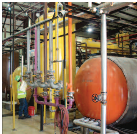
Treating cylinders are color-coded to ensure coordination between the loading process and the people in the back who oversee the treatment.
