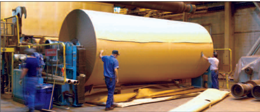
Each large reel is moved to the winder. Here, it is cut into smaller rolls for shipment to various box plants. These rolls weigh between two and three tons. This plant uses 1,000 tons of chips & 500 tons of recycled boxes to produce 1,000 tons of paper per day.
